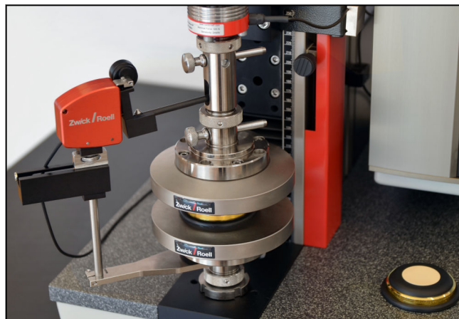
ZwickRoell displacement transducer with compression test
