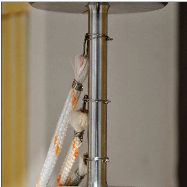
High-temperature specimen adapter for round specimens with threaded head and thermocouples
