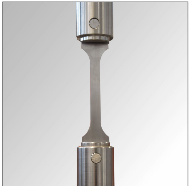
High-temperature specimen adapter for flat specimens with shoulder head and hole
