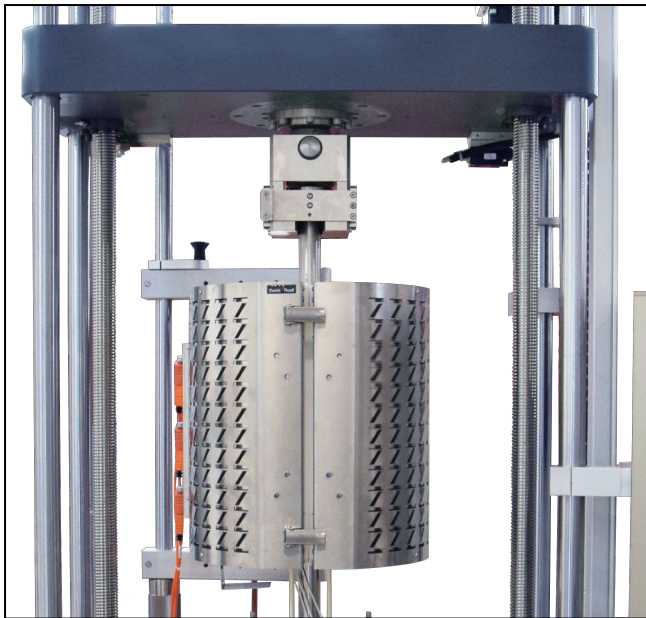
Load string and pull rod coupling in creep testing machine Kappa DS
