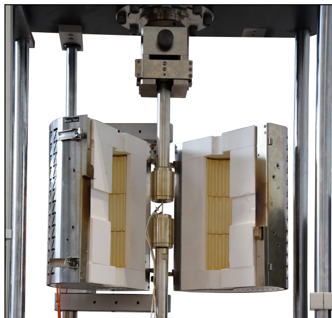
High-temperature pull rod and high-temperature furnace in Kappa SS
